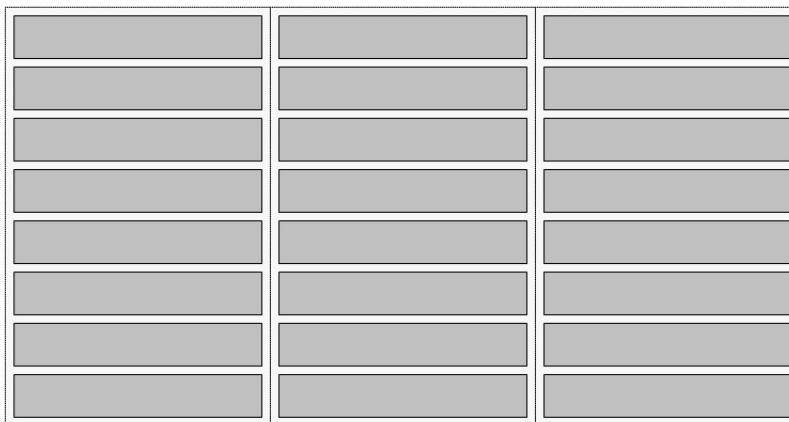
FIGURE 6. A vertical cross-section of a domain with large vertical fractures in between horizontal translations of cells with the same structure as in Fig. 1.
