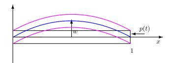
FIGURE 1. The beam; w is the displacement of the central axis.
